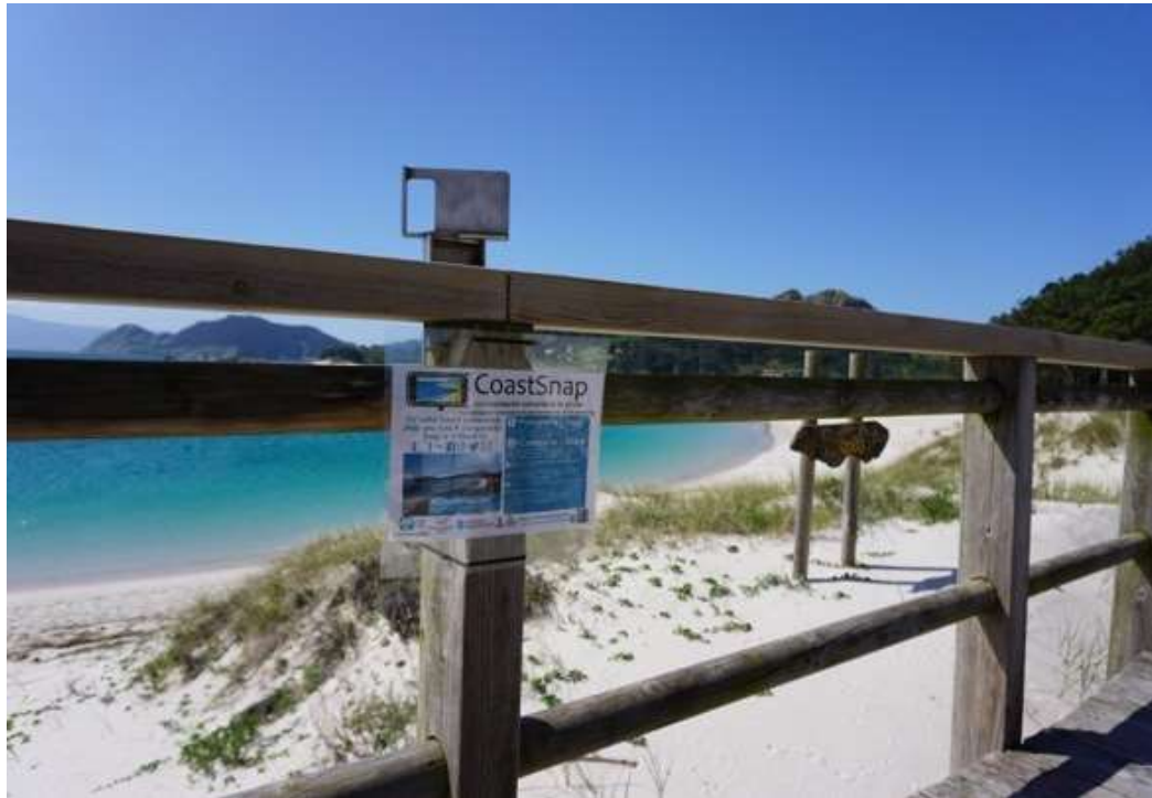
Figure 8 A CoastSnap station overlooking a coastline, including a bespoke cradle and signage explaining use.
